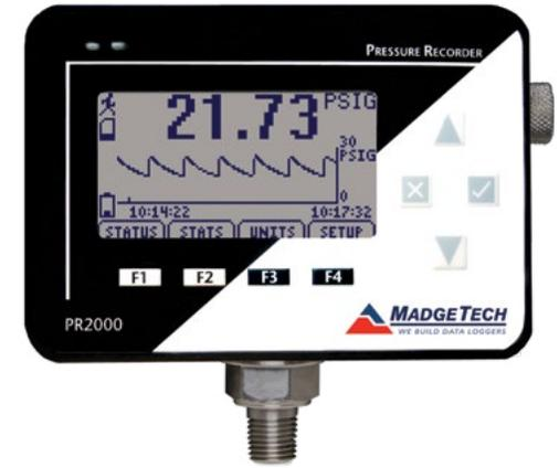
This rugged, splash-proof (IP65) device has one of the largest memory capacities of any similar data recorder on the market, logging up to 262,143 readings. The non-volatile memory will retain recorded data, even when battery power is lost. The PR2000 is ideal for applications requiring precise displayed pressure readings, such as the real-time monitoring of outdoor geothermal pipelines.
