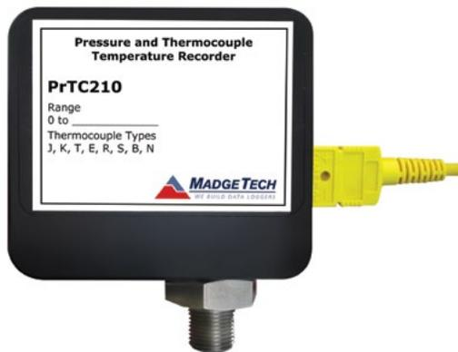
The **PRTC210** is a compact pressure and thermocouple temperature data logger with a .125 inch NPT fitting. The device accepts one thermocouple input which allows customers to measure process pressure and temperature. In addition, the PRTC210 also measures ambient temperature, allowing for a complete pressure and temperature analysis.
